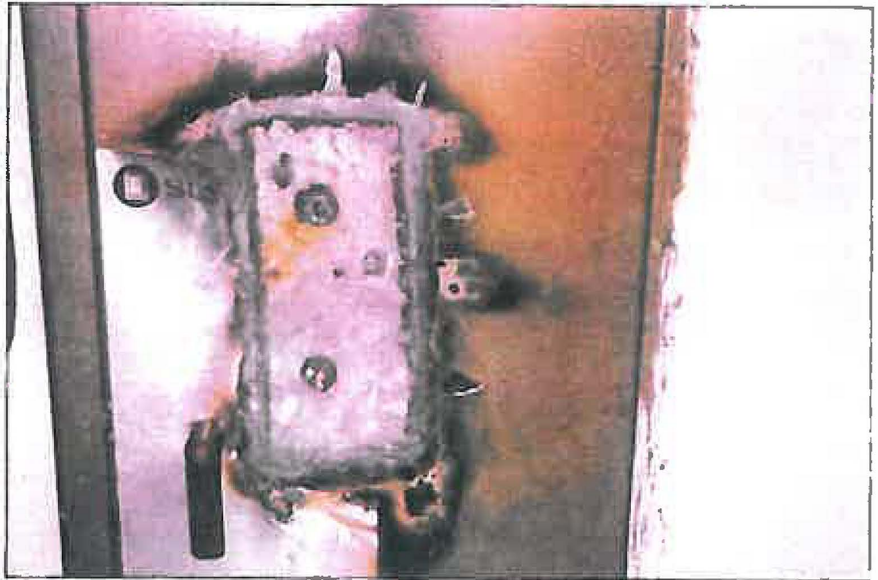
Unsuccessful: Torch and Tool Attack on the SLS Continental Mark IV (UL TL 30) Safe
