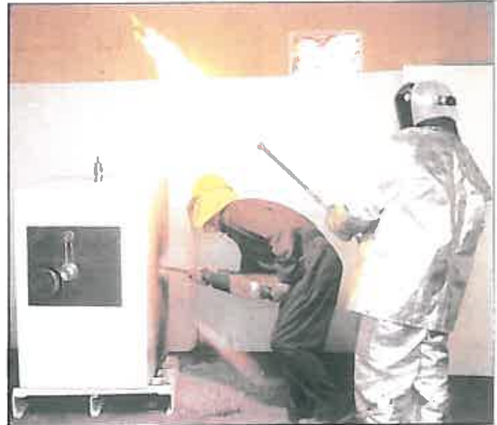
UL Combined Torch/Tool Attack.
