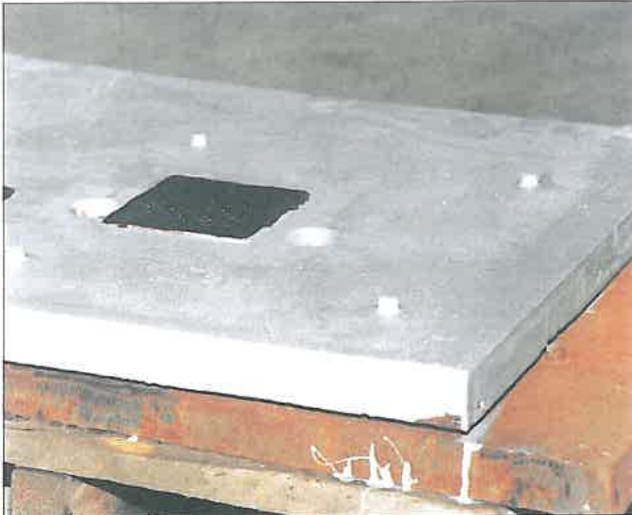
Zacalloy Stainless Steel Door Casting with Superamics.
